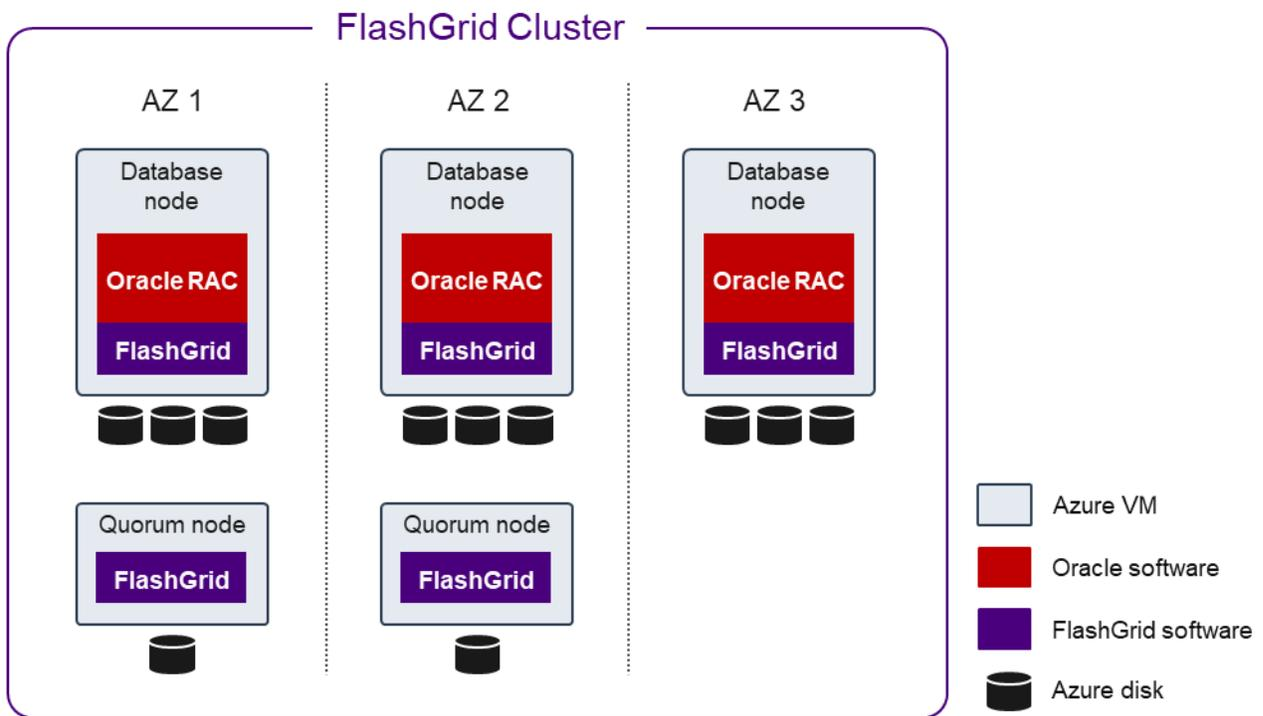
FlashGrid Cluster on Azure with three RAC database nodes
