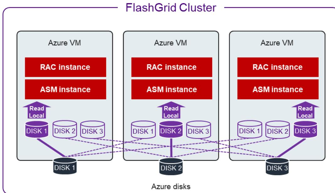
*FlashGrid Storage Fabric software architecture on Azure*
