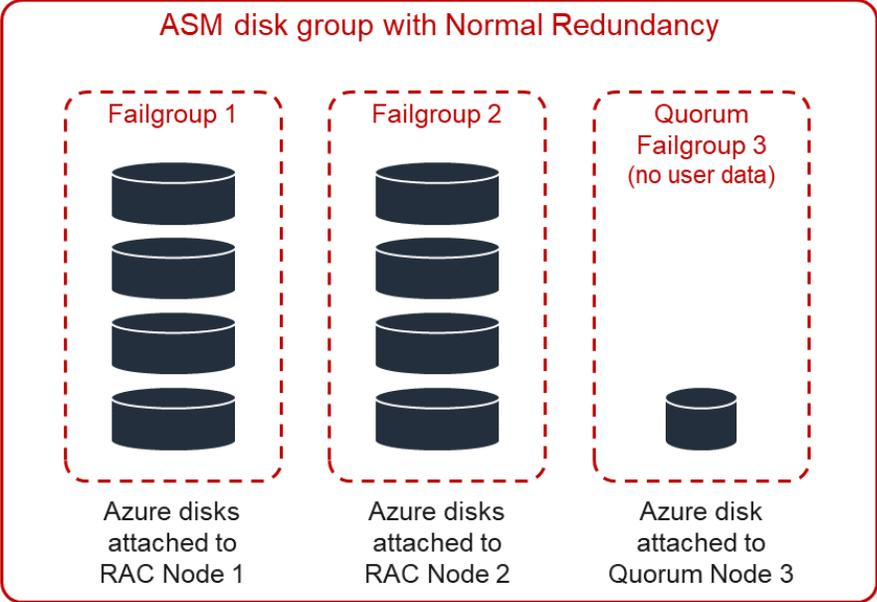
*A Normal Redundancy disk group in a 2-node RAC cluster on Azure*
