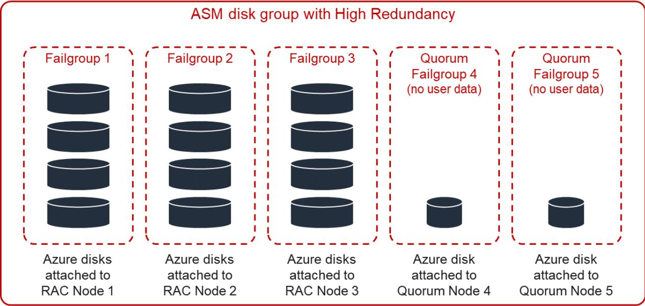
*A High Redundancy disk group in a 3-node RAC cluster on Azure*
