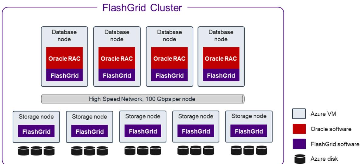
Extra-large database cluster on Azure with 4+ RAC nodes and separate storage nodes
