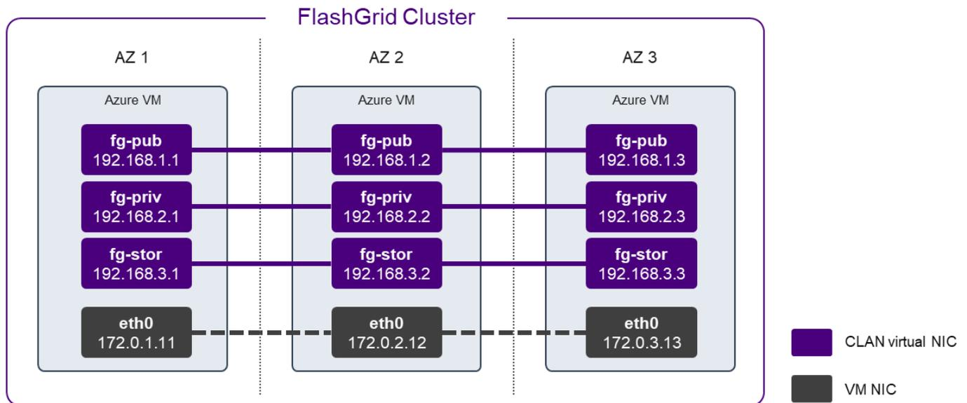
FlashGrid Cloud Area Network architecture on Azure
