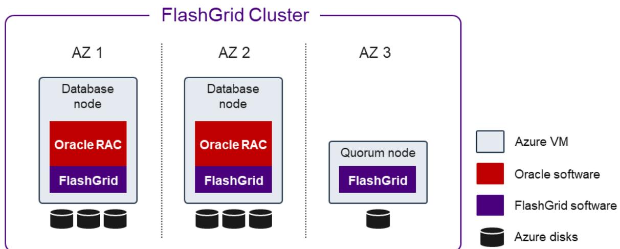
*FlashGrid Cluster on Azure with two RAC database nodes*
