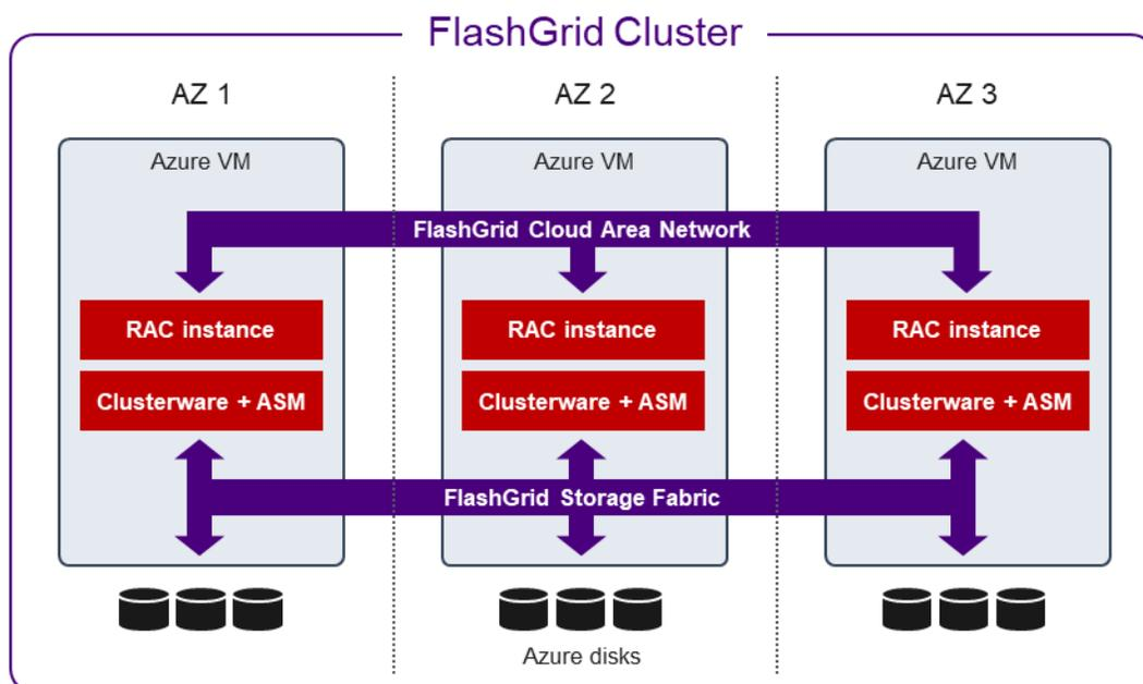
*FlashGrid Cluster for Oracle RAC on Azure: software architecture*
